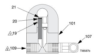
Fig. 3: Non-Circulating Setup Shown (cutaway view)
